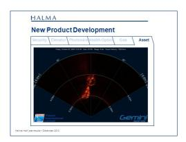
In Asset Monitoring, our sub-sea business, Tritech, has recently launched the 'Gemini' digital imaging product. Gemini provides real time, high definition imaging and can be used to inspect sub-sea objects on the seabed in low visibility conditions. The example on this side shows the image that can be seen from a vessel on the sea surface 15 metres above a well-head drilling operation.
