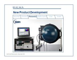
In Photonics, we recently launched our new 'TOCS' system which allows LED developers to measure the thermal, optical and electrical performance of LEDs (and their interaction with each other) in one system. This enables LED component and display developers to optimise performance and we see encouraging potential for this new system in Asia.
