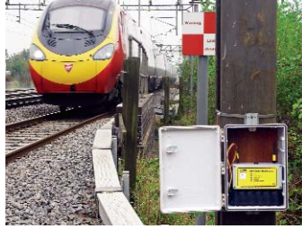
The "Best Small-Scale Innovation" at the 2006 Railway Forum/Modern Railways Innovation Awards went to Radio-Tech Limited for their Rail Temperature Monitor safety system which gives early warning of the risk of track buckling.
