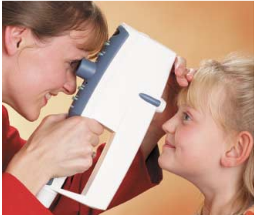
Keeler's new Pulsair Tonometer is a simple way of measuring pressure inside the eye, an important factor in the diagnosis of glaucoma.
